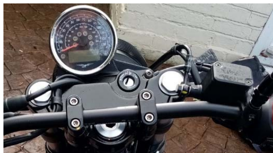
Flat Renthall bars without risers, note brake banjo angle rotated to avoid fork yoke (subsequently resolved by using 25mm
